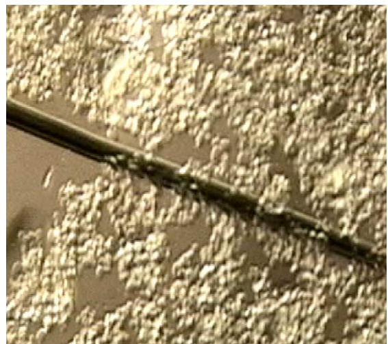
Fig. 1. Typical ice slurry crystals compared with a 500- \mu\text{m} diameter needle.
